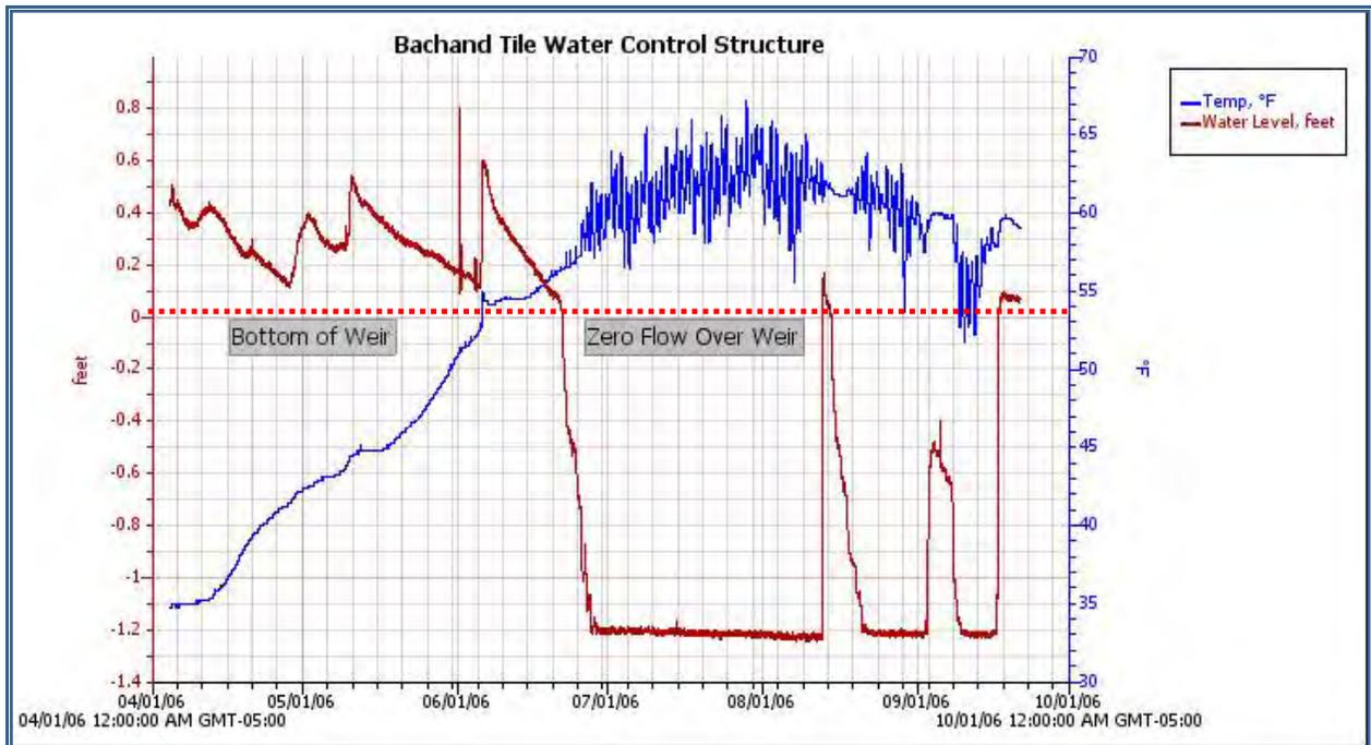
**Figure 62. 2006 Plot of the HOBO water level record at the Bachand Tile Water Control Structure**
