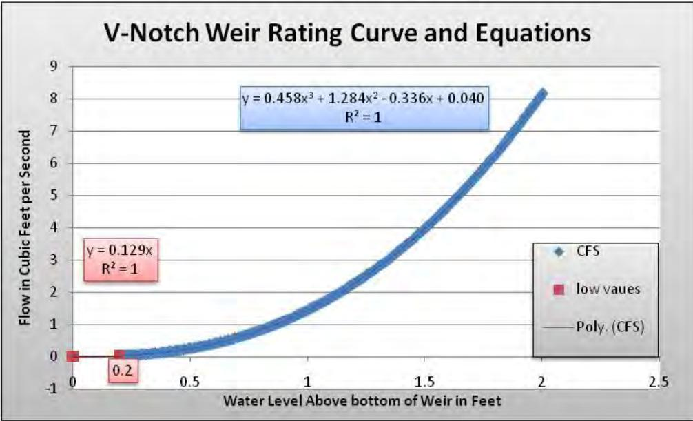
Figure 49. 60° V-Notch Weir Rating Curve and Equations
