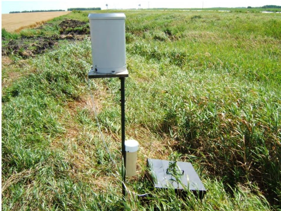
**Figure 15. Rainfall and Barometric Pressure Monitoring Equipment at the Bachand Site**
