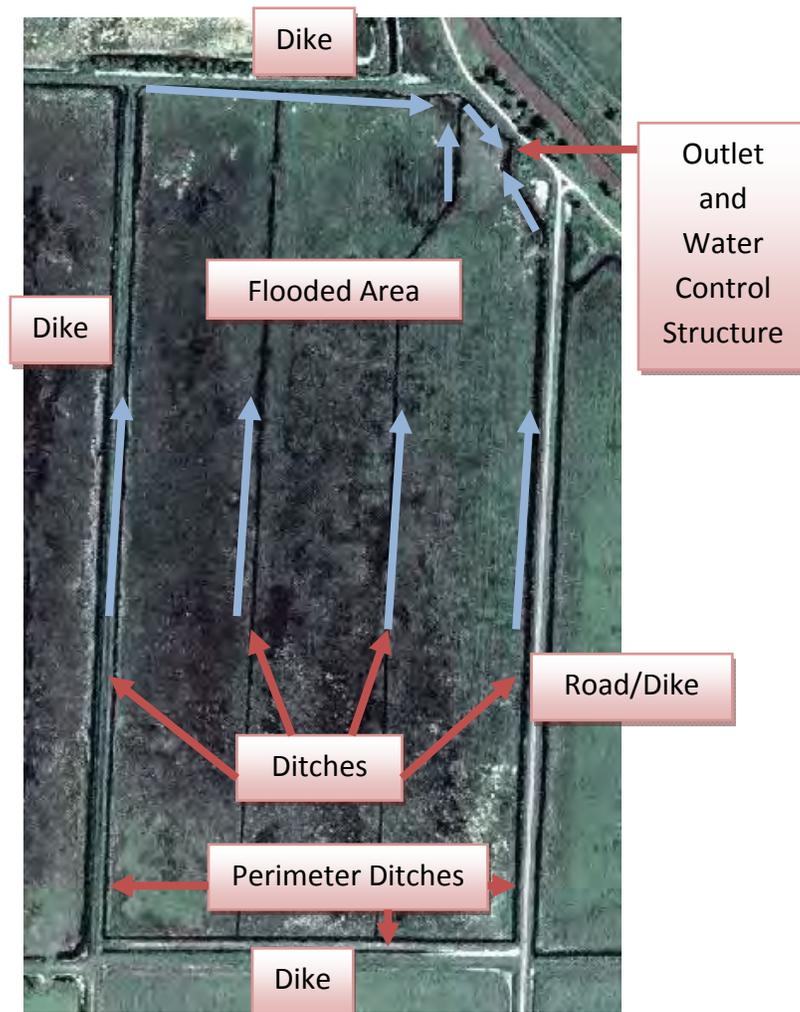
**Figure 9. Surface drained paddy aerial photo and diagram.**
