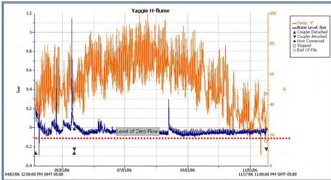
Figure 60. 2006 Plot of the HOBO water level record at the Yaggie Flume
