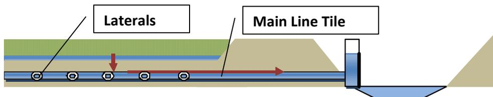
**Figure 11. Diagram of a Red Lake Nation Main Line Tile System and Outlet.**
