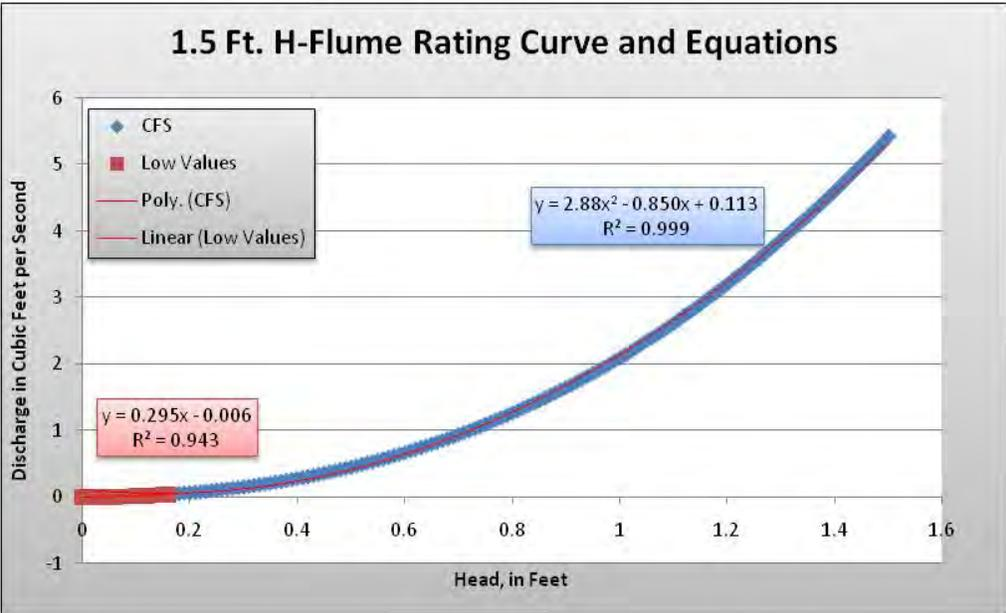
Figure 50. 1.5 Ft. H-Flume Rating Curve and Equations
