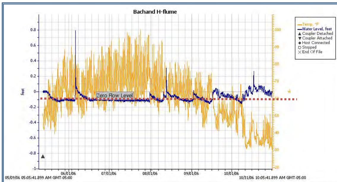
Figure 61. 2006 Plot of the HOBO water level record at the Bachand H-Flume
