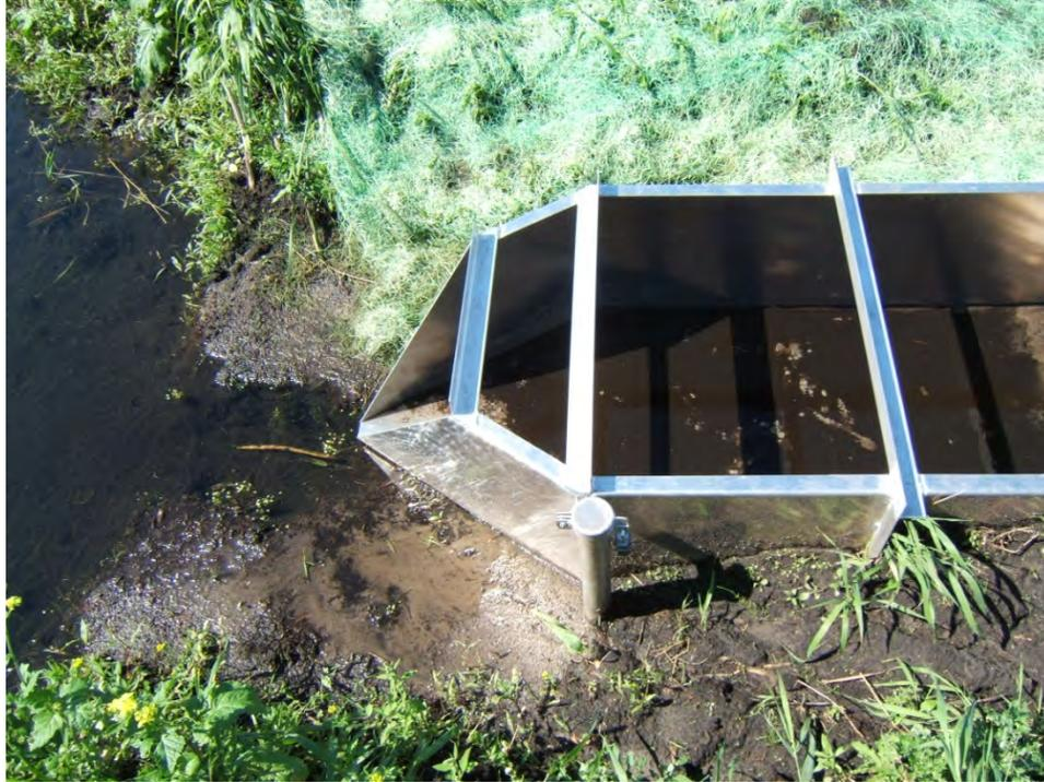
**Figure 14. H-Flume for Surface Flow Measurement at the Bachand Site**
