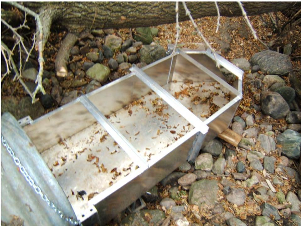
**Figure 17. H-Flume on Downstream End of Yaggie 2 Culvert**
