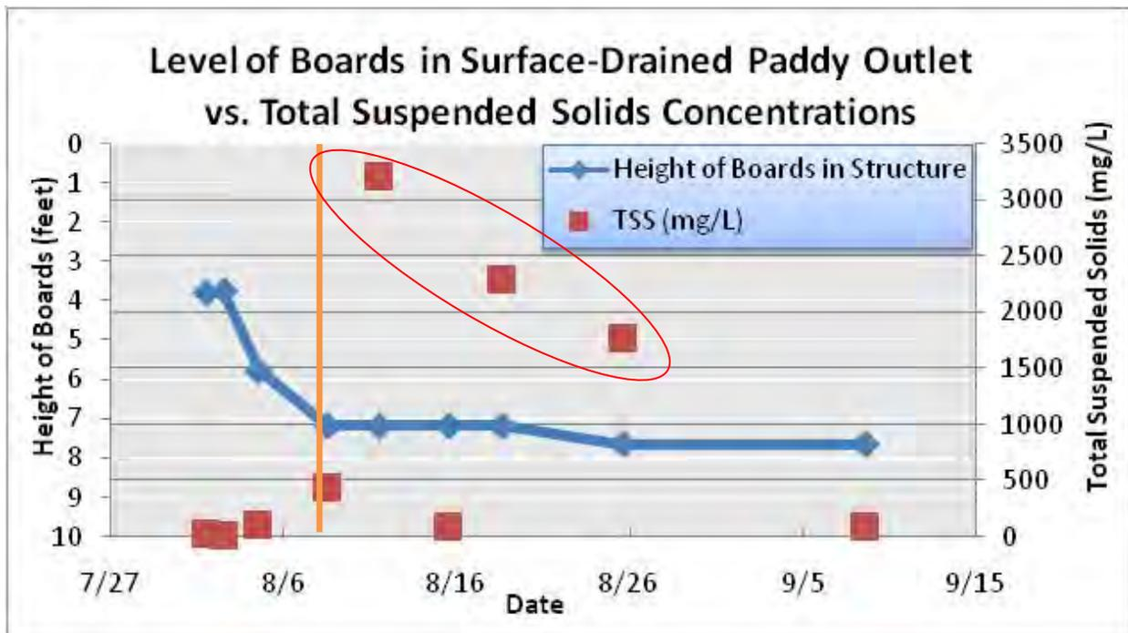
**Figure 40. Water quality problems at the surface drained paddy outlet began when nearly all of the boards were removed from the structure.**
