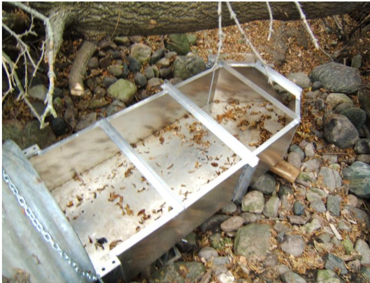
Figure 2. H-Flume Flow Measurement Structure at the Yaggie Site
