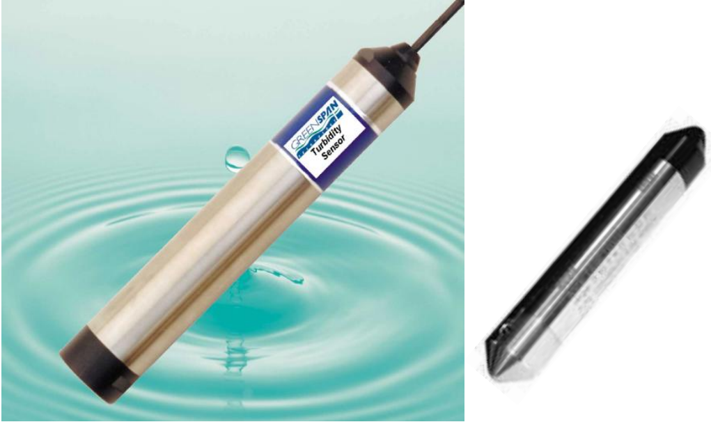
Figure 1. Turbidity - logging probe (L) and HOBO water level logging probe (R) that will be used for Project 60 water quality monitoring
