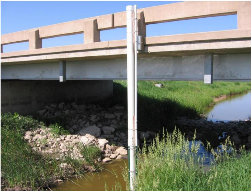
**Figure 1. Stilling Wells for Turbidity and Water Level Sensors at Stream Gauge #71 on Polk County Ditch 2**
