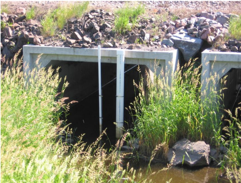
Figure 2. Stilling Wells for Continuous Monitoring Equipment at B75 (Brandt Channel at Hwy 75)
