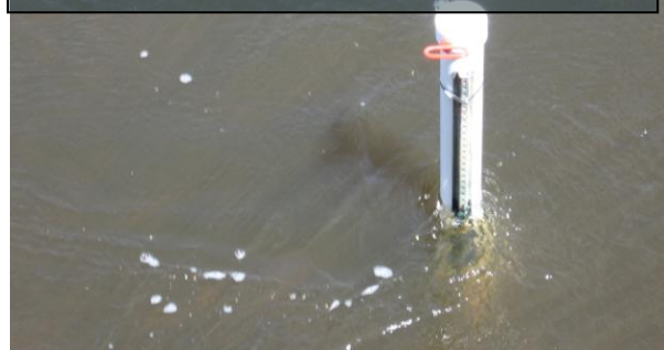
Plummer USGS Gauge Eureka Midge Dissolved Oxygen and Temperature Logging Station
