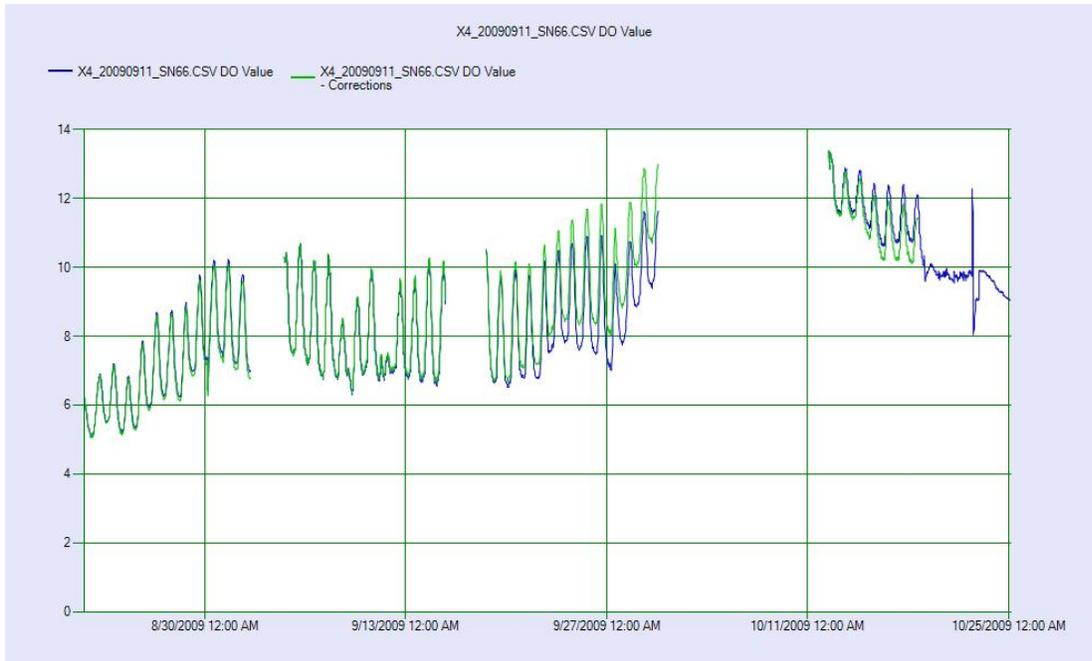
Figure 1. Dissolved oxygen record from Eureka Midges installed in the Moose River at CSAH 54 north of Grygla.
